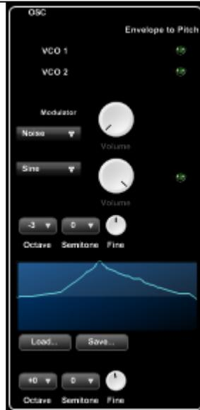
Oscillators - The two green led buttons at the top switch on/off the 'envelope to pitch' controlling all of the oscillators 1-8 and 9-16 - the lower ADSR - see later.
