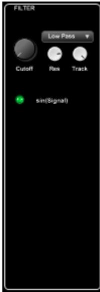
This section applies a filter to the audio output. You can vary the cutoff, resonance and keyboard tracking. Filter types are low pass, high pass, band pass, band reject and peaking.
